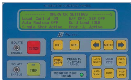
Operator control panel
